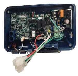
3 Locate the terminal at the main power input.
