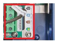
B Remove the brown wire at position L2 from the terminal at the main power input;
