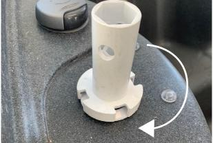
10 Screw on the faceplate and keep one hand on the jet underneath to prevent it from moving. Tighten with the wrench tool and reinstall the top of the waterfall.
