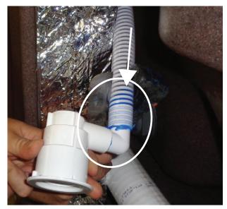
7 You must cut the hose just after the 90° adaptor. Please carefully notice the angle of the jet because when you will install the new one, it must be in the same direction;
