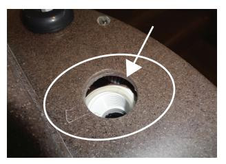
9 Replace the jet in the right place. Insert the flat gasket between the spa wall and the jet. Place the gasket with the groove facing the jet. Be sure to place the jet at the same angle as when you removed it;
